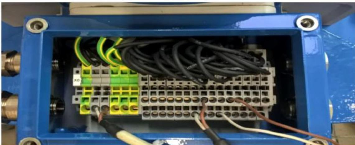
*Fig. 8.19: Connection of the RS 485-2 (22 +, 23 -) at the USM GT400*
