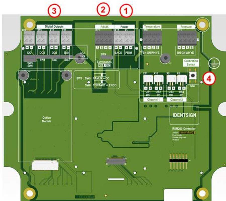
**Figure 11: Internal terminal assignment of the RSM 200**
