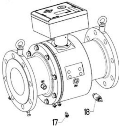
**Figure 64: General version with pressure transducer**
