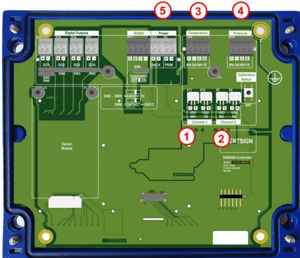
**Figure 10: Internal terminal assignment of the RSM 200**
