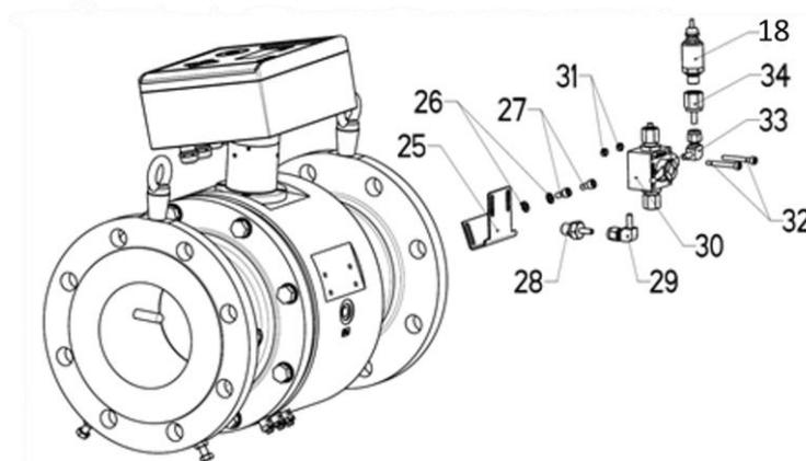
**Figure 68: Version with 3-way valve with pressure transducer**
