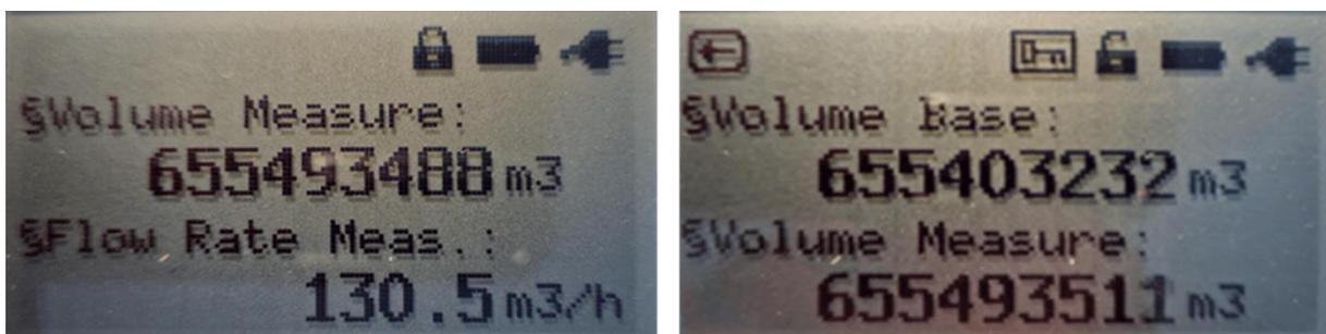
**Figure 31: Main/start display (without / with quantity transformer)**
