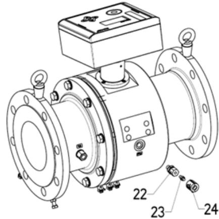
**Figure 65: Version with Pressure port Ø 6 mm**
