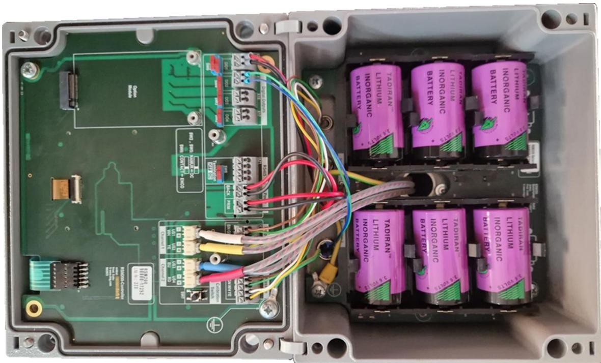
**Figure 17: Location of the battery compartment**
