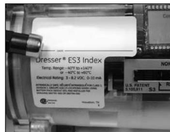
Figure 2 - Swipe magnet across the "swipe line" to change the screen displays
