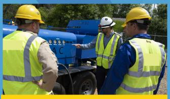
4.) ZEVAC pumps gas (and liquids) out. Monitor and wait for auto-shutoff
